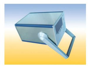
systems into Racks. DiVar case from Intermas fits in the best way to these requirements. As bases Aluminium die cast corner profiles allow variation of every dimension as desired. The construction principle allows easy mounting of chassis plates, PCB's or additional components by threaded inserts shoved into special slots within the corner profiles. Several kind of sheet material can be used for panelling: aluminium, steel, stainless steel or plastic. The panels will be
