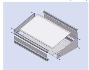
As bases Aluminium die cast corner profiles allow variation of every dimension as desired.
