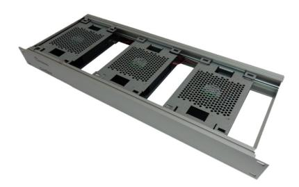
The basic construction consists of a front panel, a back panel and two side stripes. This 19" frame can take in up to four fans in width, each being preassembled as a single module. The modules are composed of two mountingplates which include one fan. The fan itself is linked to the mountingplate via plug-in connections and mortise joints; there are no other screw connections necessary.
