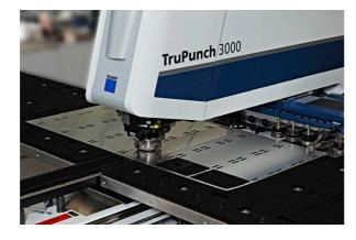
Front and rear panels with holes, openings and cut-outs are also available in punched versions, up to a material thickness of 3 mm. On our punching and nibbling machines we can produce cut parts, perforations, holes and carry out countersinking, reshaping and embossments, at low cost and in a single manufacturing step.
